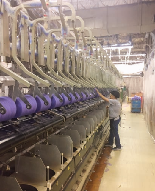
National Spinning employee Melinda Williamson processing acrylic craft yarn on a Volkmann twister.
